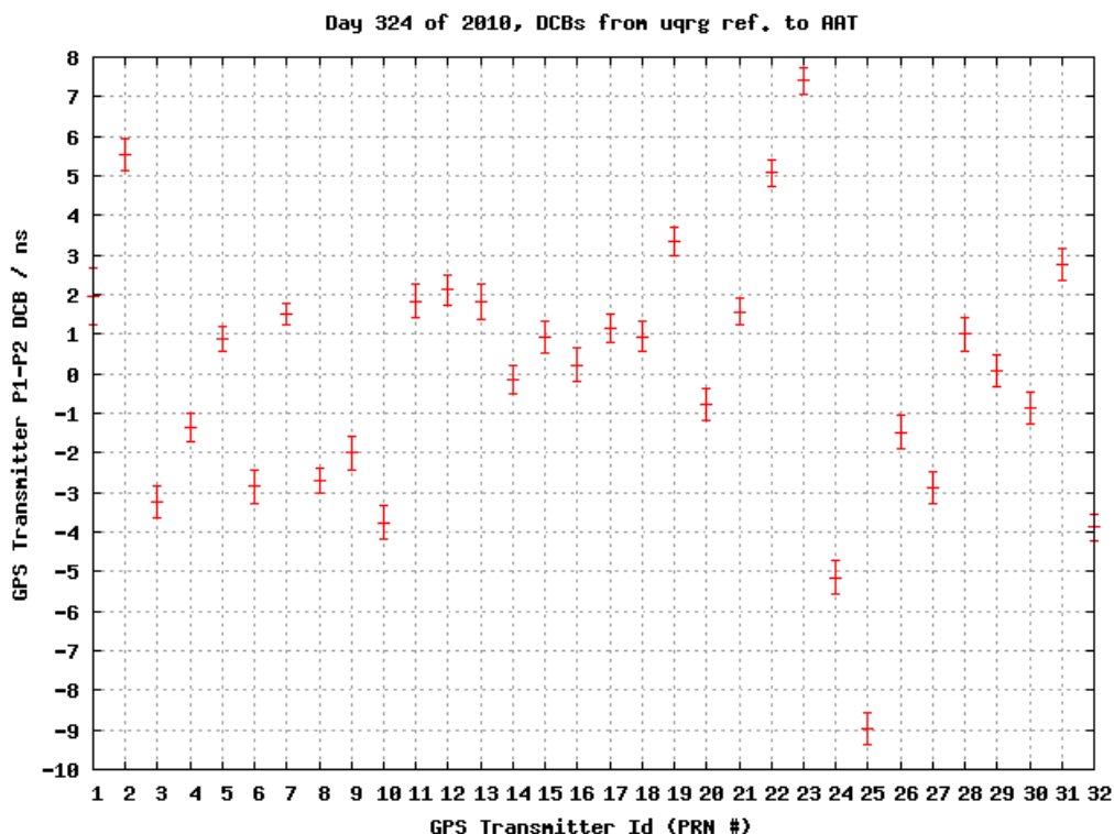
Figure 3: Example of GPS transmitter DCB values associated to TDCBs-TOMION UPC external products for day 324 of 2010 (file tdcbs-uqrg.2010.324.mutd.gps.snapshot.gif , see Table 4 for details).
